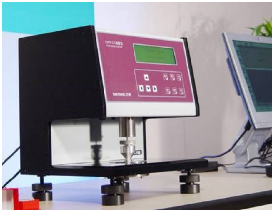
Fig.1 Labthink CHY-C1 Thickness Tester
